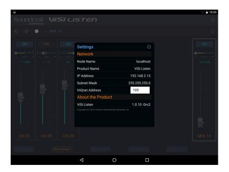
In the above Example the HiQnet address of the device was 105 but will be changed to 12. This number then needs to be entered into the console's Device ID column as well:
