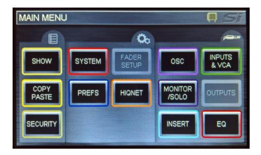
Select the 'SYSTEM' Menu and confirm the console has a valid IP and HiQnet address
