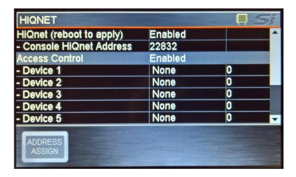
Next it is necessary to set a Device ID in the right hand Column of the Si HiQnet menu page (on previous page) which matches the HiQnet address of the mobile tablet device you are using with ViSi Listen. Each musician must have a different HiQnet address set on their mobile device, this is done by accessing the Settings page in ViSi listen:
