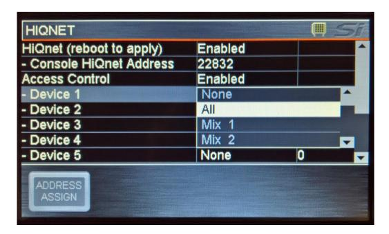
Here we have selected Mix 1 for access by the ViSi LIsten device which has HiQnet address 12 assigned.
