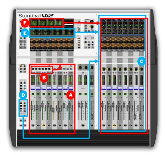
The 8 Master section faders A are dedicated to control of VCAs and Bus masters, as on the Vi4 and 6. The assignments for these faders are controlled by a set of Output Fader Page buttons B within this section, and can be customised using the associated Fader Page Setup button.
