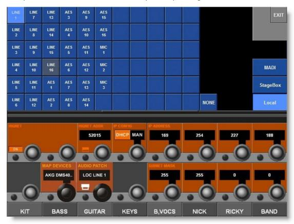
The patching matrix allows all of the physical input connectors available within the Vi system to be seen and the relevant connector to be chosen to correspond to where the currently selected microphone is connected.
