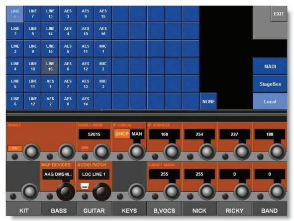
The patching matrix allows all of the physical input connectors available within the Vi system to be seen and the relevant connector to be chosen to correspond to where the currently selected microphone is connected. The chosen connector is shown in bright blue highlight, whereas connectors that are already associated with other AKG devices are shown as greyed-out.
