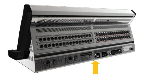
Important! The HiQnet port on early Vi1 consoles (serial numbers lower than 30210956) is only able to drive short cable lengths, max recommended length 1 metre (3 feet). Therefore use a network switch positioned close to the rear of the console to extend the cable length if required.
