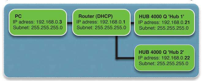
**EXAMPLE:** The following example shows a HiQnet system with a PC running System Architect, a router (DHCP turned off) and one HUB 4000 Q. The PC is in the right subnet but it's IP address is configured wrong. System Architect will not discover the HUB 4000 Q because there is no proper network connection between the PC and the HUB 4000 Q. The IP address of the PC should be **192.168.0.10**. Then the PC would be configured right.
