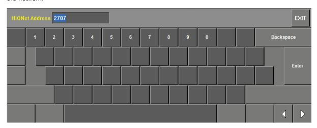
To set the HiQnet address, press the button within the HiQnet Address Vistonics control (see screenshot on previous page). A keyboard will be opened which will allow the default address to be edited.
