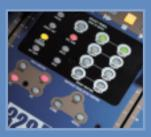
The 328XD's Snapshot Control Panel is used to store and select up to 100 snapshots, in which every digital parameter is instantly recallable. The Select Panel also provides swift and intuitive routing and assignment for the selected channel.
