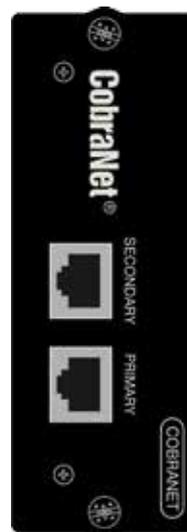
This card allows sending and receiving of up to 32 audio channels to/from a CobraNet® network. DIP switches on the card allow setting the number of input or output channels seen by the console. Default setting is 32 output and 32 input channels. CobraNet cards used in Soundcraft consoles must operate as the conductor of the CobraNet system.
