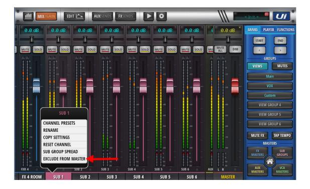
In certain situation where the user may want an output only patched to a Matrix or the ability of just hearing FX are needed without the main channels, excluding a group from the master output would be necessary.
