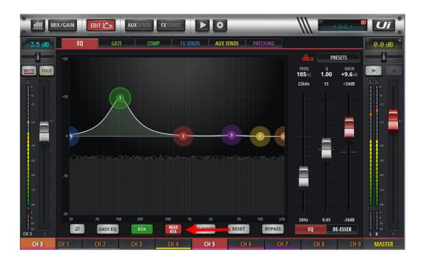
Clicking the HOLD RTA button will create and hold an outline of the RTA on the screen which will then allow you to see the changes in the RTA when EQ is applied. This also forms part of the next section which will then enable the user to view a channels RTA in a master EQ page.
