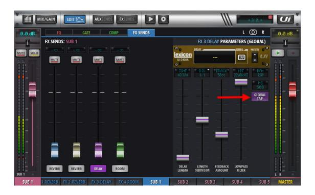
Each delay can now be linked to the tap button on the GUI, this can be turned ON or OFF allowing the user to control 1 or both delays.
