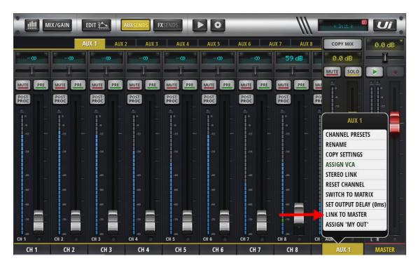
The AUX or MTX send master will now follow the Master level. This is often used when sending a separate mix to a subwoofer from an AUX or wanting to control delay speakers or sends with the master level as well.
