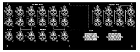
The BUS/LINKING INPUTS are on female XLRs. They are all balanced inputs at +4dBu, and are injected directly onto the appropriate bus at unity gain.
