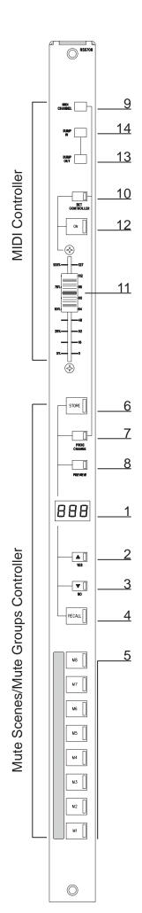
dump. When you do press the DUMP IN button the 7-segment display shows three flashing bars, which stop flashing while incoming MIDI data is being received. At the end of the dump, the RAM is protected again, and the 7-segment display returns to the scene number display. To abort the DUMP IN procedure (e.g. if no data is received), the DUMP IN button may be pressed while the flashing bar is displayed. The 7-segment display returns to the scene number display.
