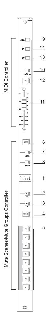
information which will turn the appropriate cuts on and off, it will also receive Program change information to select mute scenes. This channel will also transmit Note On and Note Off data from the cut switches: note that if the MIDI CHANNEL is set to ANY no Note On or Note Off data will be sent.
