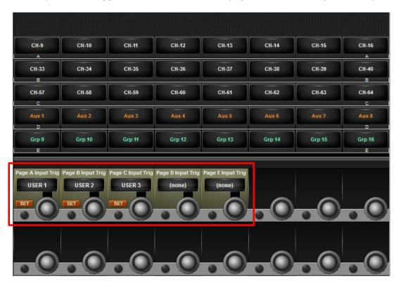
The trigger button has the effect of providing a link between Input Fader page button and Output Fader page button as shown below:
