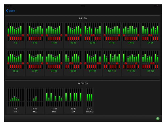
Touching any section of 8 meters will immediately switch the view to the fader panel for those channels or busses, allowing an alternative way to move from one set of channels to another without having to scroll the fader panel.
