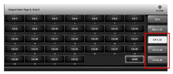
When a fader page strip is selected for assignment, the Assign page shown above appears. In the tabs on the right hand side of this screen, Input channels can now be found and the relevant bank (1-32, 33-64 or 65-96) and the required channel selected.
