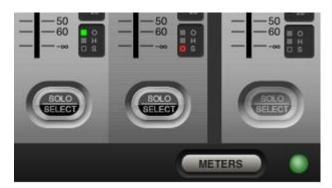
The Meters page itself displays an overview of up to 128 input channels, 32 busses and LRC masters, together with the corresponding Gate-closed and Compressor gain reduction indication.
