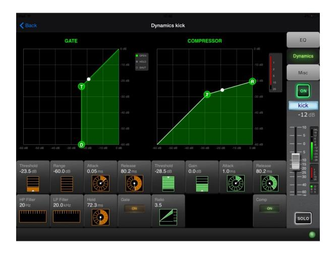
The updated dynamics page now includes Gate open/hold/closed indication, compressor gain reduction metering and the selected channel or bus strip shows the current signal level.
