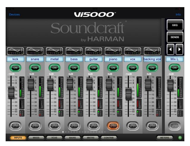
New Fader panel view showing metering for channel and bus signal levels, plus gain reduction and gate open/hold/closed indication.
