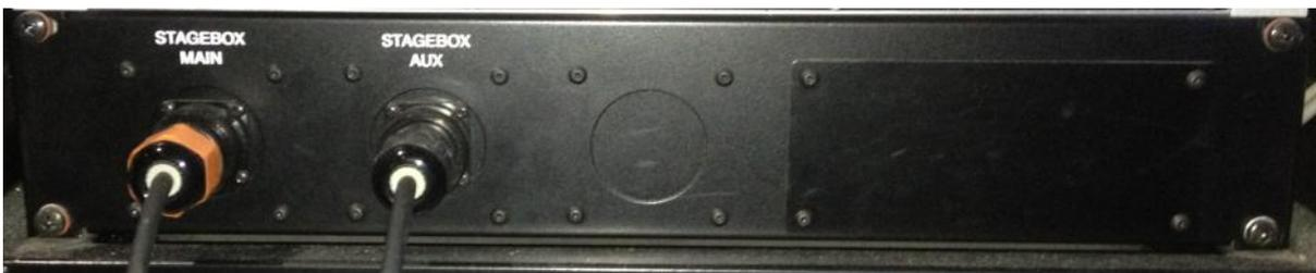
As the Vi1 has its 'local rack' built internally to the console, the flight case that can be purchased feature pre-cut holes at the rear on both sides for panel mount Fibrecast connectors. A part which consists of the heavy duty panel mount Fibrecast connector, link cable & optic SC connector is available for purchase to allow use of a Vi1 with a Vi stagebox (The part order number is BF10.947010). Two would be required for a redundant link.
