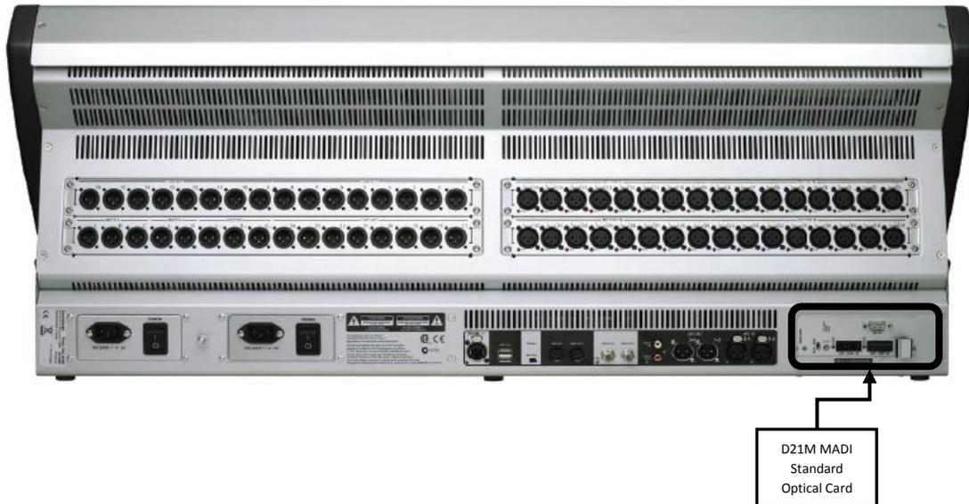
The 'two card width' option slot on the rear of the Vi1 accepts a number of optional cards. The most common card used is the standard MADI card (both optical & CAT5) - Remember the MADI card takes up both card slots as it is 'double sized'. This card allows connection to external MADI equipment such as multi track recording/playback devices or Soundcraft stage boxes.
