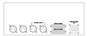
The MONITOR/COMMS D-type connector routes signals to the Monitor Selector PCB ( see the Meterbridge connector list on the previous page for pin details).
