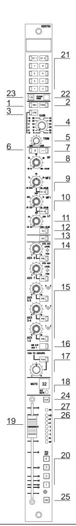
add, or subtract, an offset to the level set by the module's fader: this is done by use of the VCA GRP 1, 2, 3 & 4 switches.
