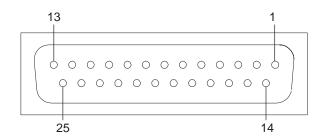
The pin-outs of the various D-types are given below.
