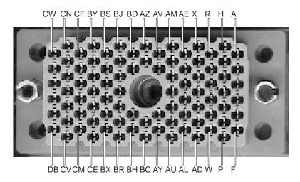
The pins are listed in circuits below - the circuit functions for each EDAC are shown on the following pages.
