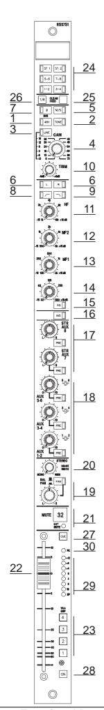
it down for. If you press and release within approximately 0.5 seconds the button will latch. If, on the other hand you press and hold for more than 0.5 seconds then the cue will not latch.
