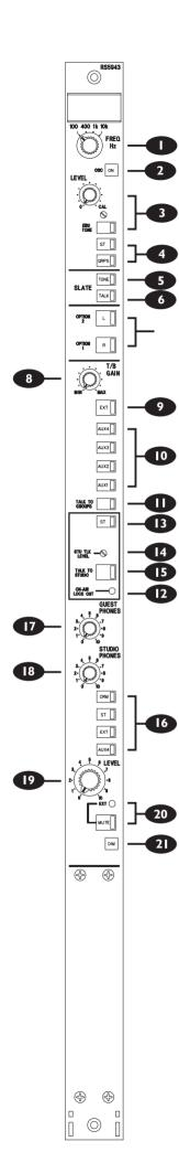
When the switch in question is released the talkback output carries, depending on link settings, either no signal or the signal from the EXT CUE contacts which are also available on the Comms Module EDAC. When the switch is pressed the appropriate output carries the console Talkback signal.
