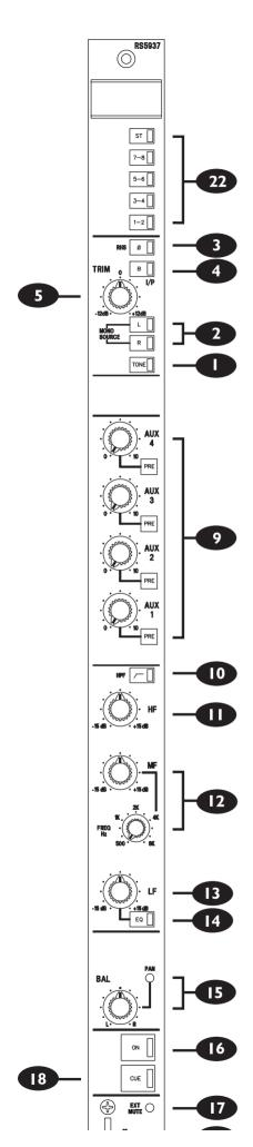
When the input is in line level mode and the CUE switch is pressed, this will (optionally) trigger the remote start/stop facility which has two sets of relay contacts, available via the rear panel D-type connector. These relays can be set to either latching or pulsed operation via internal jumpers, enabling most types of machines to be remotely started and stopped.
