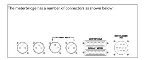
The MONITOR/COMMS D-type connector routes signals to the Monitor Selector PCB ( see the Meterbridge connector list on the previous page for pin details).
