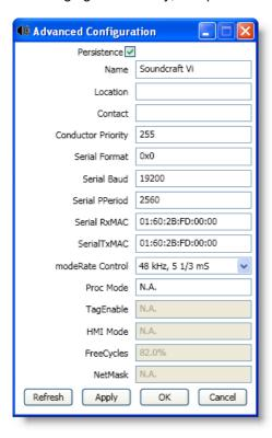
The **Advanced Configuration** dialogue box is used to set the Latency and Sample rate of the CobraNet card (this is the parameter called 'modeRate Control')
