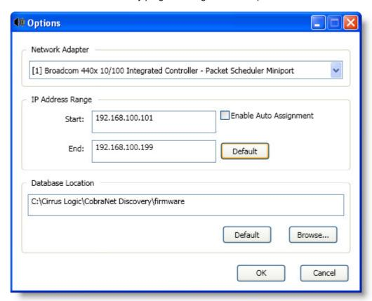
In the top section of the dialogue, select the network controller that your laptop is using for the Ethernet port you have connected the module to.
