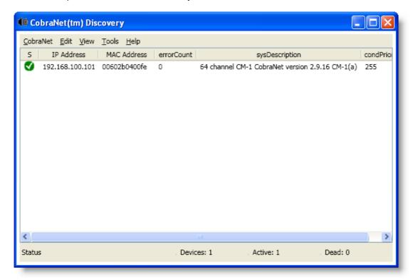
4. To configure the CobraNet card, click on the CobraNet device to select it, then choose Tools/Configure – or just double-click the device.
